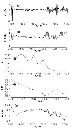
Fig. 1 Time history of flight variables for Transport A in severe atmospheric turbulence during the descending phase in transonic flight
