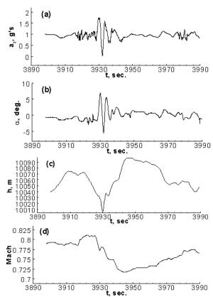
Fig. 2 Time history of flight variables for Transport B in severe atmospheric turbulence at the altitude around 10,050 m in transonic flight
