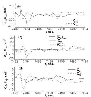
Fig. 5 Time history of main longitudinal and lateral-directional oscillatory derivatives along the flight path
