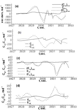
Fig. 6 Time history of main longitudinal and lateral-directional oscillatory derivatives for Transport B along the flight path
