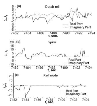
Fig. 8 Eigenvalues of lateral-directional modes of motion for Transport A
