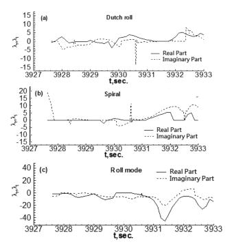
Fig. 10 Eigenvalues of lateral-directional modes of motion for Transport B
