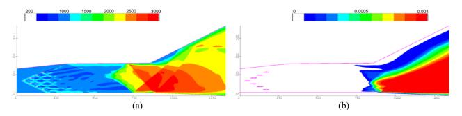
Fig. 1. Static temperature (a) and NO mass fraction (b) fields for model combustor in the case  $T_0$ =1100 K
