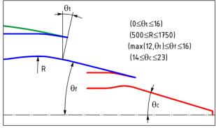
Fig. 1. Control geometrical parameters for bypass nozzle
