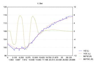
Fig. 4. Velocity and angle of slide simulated and experiment values match (on-board measuring system functioning correctly)
