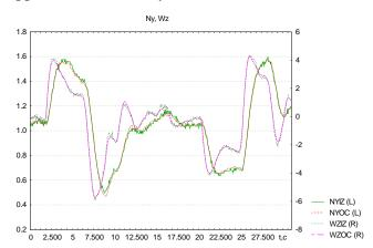
Fig. 9. The match between experiment and simulated values of normal overload  $n_{_{\rm V}}$  and pitch angular velocity  $\omega_z$
