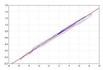
Fig. 8. The  $c_y(\alpha)$  estimates after correction of the lag in the angle of attack measurements
