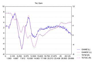
Fig. 3. Angles of pitch and roll simulated and experiment values match (on-board measuring system functioning correctly)
