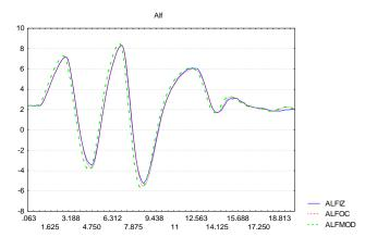
Fig. 2. The lag detection in the angle of attack measured values
