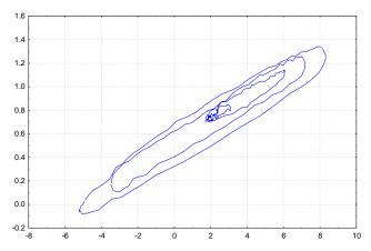
Fig. 7. False aerodynamic hysteresis of  $c_y(\alpha)$  estimates caused by the lag in the angle of attack measurements
