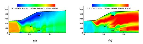
Fig. 9. Mach number (a) and temperature (b) fields for the combustion in pseudo shock
