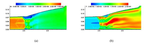
Fig. 8. Mach number (a) and temperature fields (b) for iso-Mach combustor
