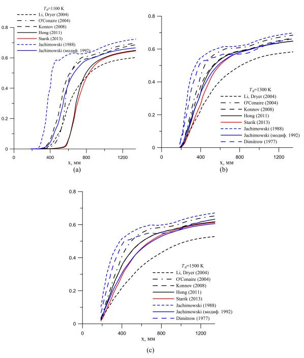
Fig.7. Combustion efficiency  $\eta$  as the function of the duct length (a) –  $T_0$ =1100 K, (b) –  $T_0$ =1300 K, (c) –  $T_0$ =1500 K
