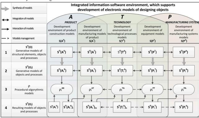
Fig. 2. Scheme of relations between parallel engineering models.
