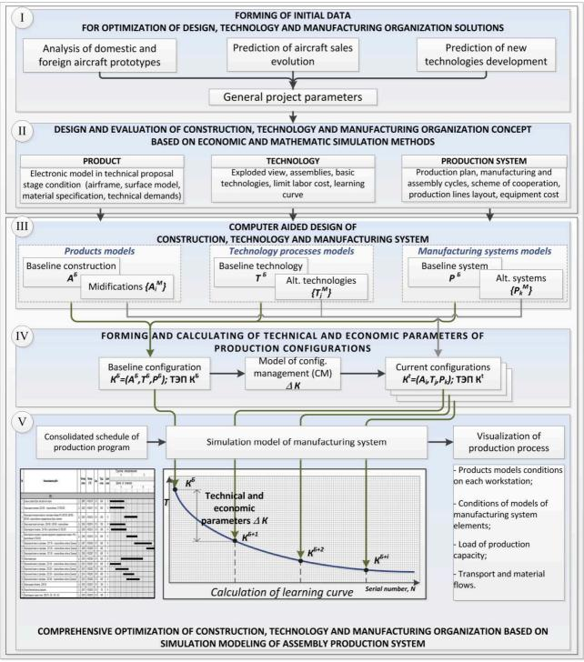
Fig.1. Scheme of making and optimization of construction, technology and manufacturing organization decisions of assembly production.
