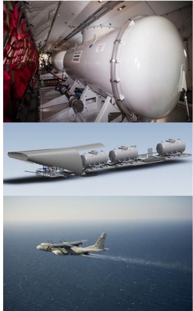
Fig.1 The OSD system integrated into the Airbus DS C295 aircraft cargo bay (upper). Schematic view of the OSD system (middle). Spraying operation (bottom)
