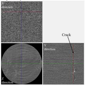
Fig.16 Reconstructed image of three direction
