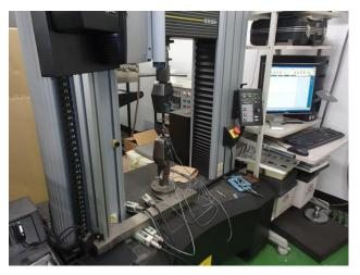
Fig.4 Tensile test on CF3 sample
