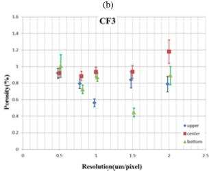
Fig.12 Relationship between Porosity and Resolution (a) CF1 (b) CF2 (c) CF3
