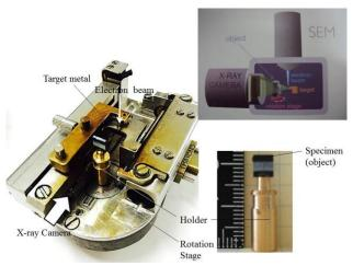
Fig.2 Specimen on a metal holer
