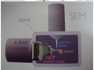
Fig.1 Mechanism of Micro X-ray CT in SEM
