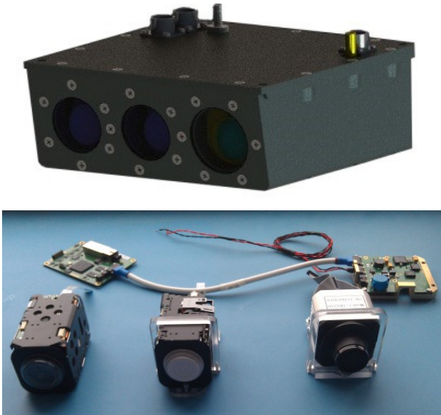
Fig. 1. The model of EVS optical unit (top) and the photo of EVS sensors (bottom)
