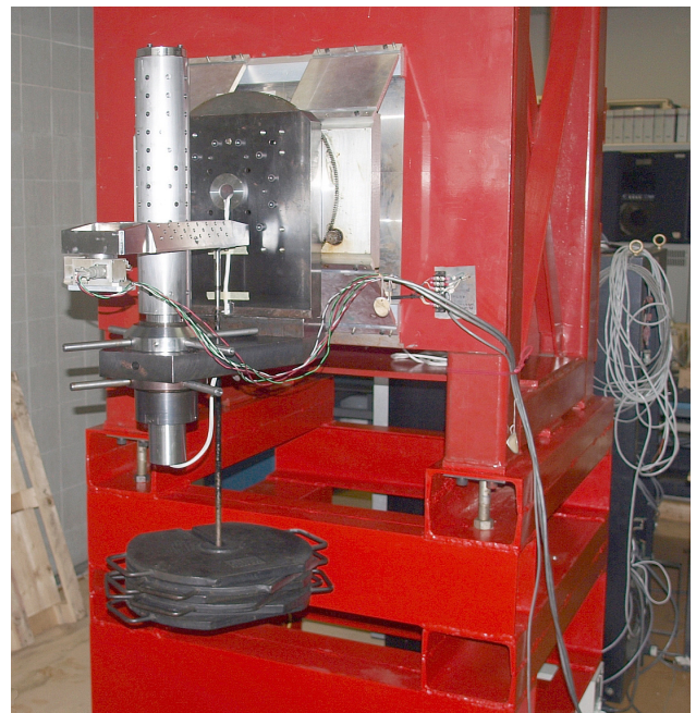
Fig. 9. Calibration of a 9 kN internal wind tunnel balance on the upgraded calibration rig in VTI; simultaneous application of axial force and pitching moment.
