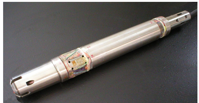
Fig. 6. The 40\text{ mm} VTI-produced high-stiffness monobloc balance with semiconductor strain gauges on the axial-force component
