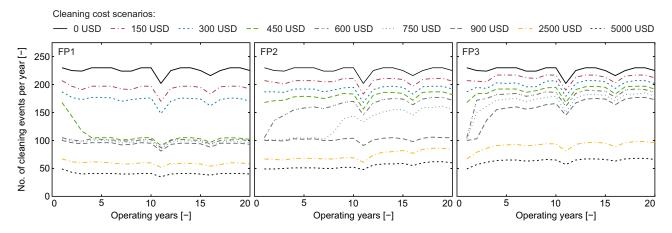
Fig. 12 Change of cleaning intervals per year as a function of fuel price and cleaning cost (contamination scenario 1, route-mix operation; the drop of cleaning events after 11 operating years originates from the D-check).
