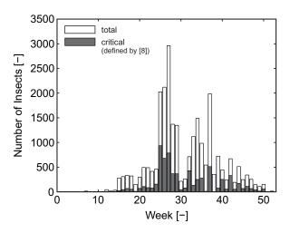
Fig. 3 Number of insect debris on the wing leading edge over a time period of one year [8].
