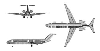
Fig. 2 DLR's concept for a FSW-NLF aircraft (designed with PrADO [20, 21]).
