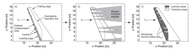
Fig. 4 Process of modeling the impact of insect contamination on available laminar area.
