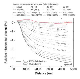
Fig. 8 Impact of insect contamination on fuel efficiency (bulging of the fuel saving curves for missions around 1,000km originates from different optimum initial cruise altitudes).
