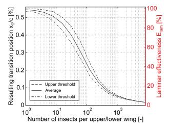
Fig. 6 Trend of laminar effectiveness and resulting transition position depending on the number of insect debris on one wing side (here  $E_{lam}$  is related to only one wing side (upper or lower wing)).
