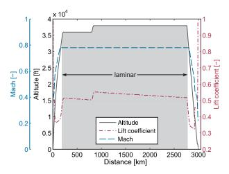
Fig. 7 Trajectory for a 3,000km mission with conditions of altitude, Mach number, lift coefficient and laminar state.
