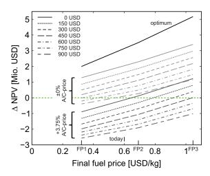
Fig. 17 Change of  $\Delta$ NPV with increasing cleaning cost per even and aircraft price (route-mix operation, contamination scenario 2).
