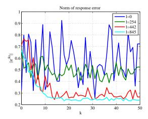
**Fig. 8** Norm of response error using modified response error sampling in Case 1.
