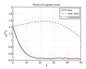
**Fig. 4** Norm of response error using three kinds of impulse responses in Case 1.
