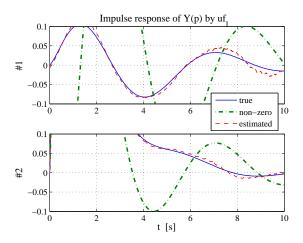
**Fig. 3** Impulse response of Y(p) by  $u_{f_1}(t)$ .
