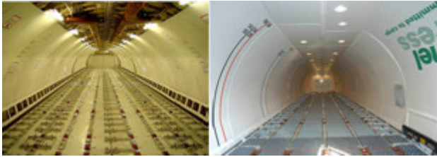
Figure 24: Cargo loading system B747-400BDSF (LH), B737-400BDSF (RH)
