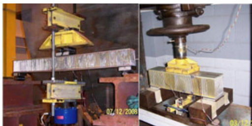
Figure 34: 9g rigid barrier shear & bending tests
