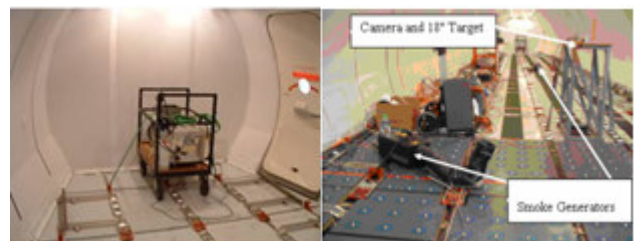
Figure 18: Smoke detection and penetration tests
