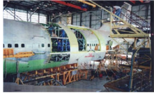
Figure 7: B747-400BDSF cargo door cut-out
