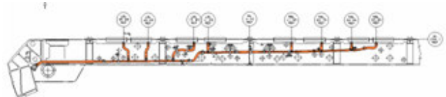
Figure 31: B737-400BDSF main deck floor drain
