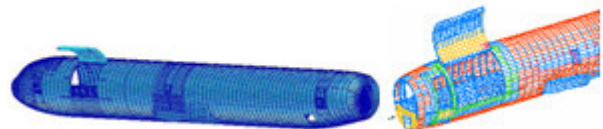
Figure 8: B767-300BDSF / B737-400BDSF finite element model (FEM) with MDCD open
