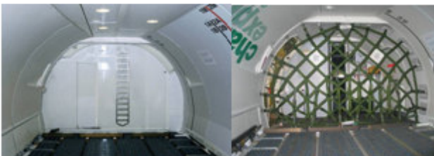
Figure 33: 9g rigid barrier and 9g safety net
