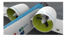
Figure 5: Electrical Ducted Fan
