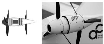
Figure 1: Electric motors configuration and air inlets visualization
