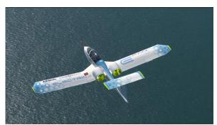
Figure 8: E-Fan 1.0 crossing the Channel
