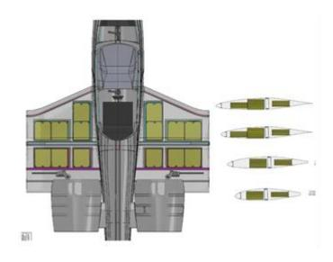
Figure 6: Battery Installation
