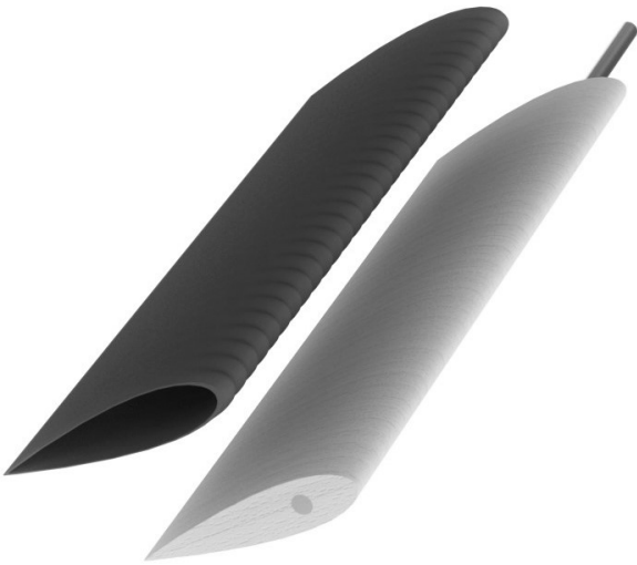
Fig. 1. CAD models of NACA0021 baseline wing and tubercle sleeve.
