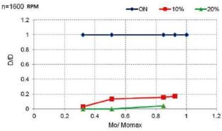
Fig. 10. Relative changes in smoking engine as a function of the relative load changes for different fuels at a rotational speed 1600 rpm
