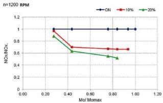
Fig. 6. Relative changes in the concentration of NOx in the engine exhaust gases as a function of the relative load changes for the various fuels for speed of 1200 rpm
