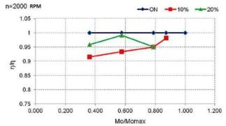
Fig. 5. Relative changes in the overall efficiency of the engine as a function of the relative load changes for different fuels, for speed 2000 rpm
