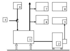
Fig. 1. The dynamometer test engine rig scheme: 1 – engine, 2 – dynamometer, 3 – supply of diesel fuel, 4 – supply of water fuel microemulsion, 5 – gauge of rotational speed and torque, 6 – exhaust gas analyzers, 7 – opacimeter, 8 – gauges of atmosphere state
