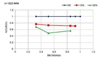
Fig. 7. The relative changes in concentrations of NOx in the exhaust of the engine as a function of the relative load changes for different fuels for rotational speed 1600 rpm
