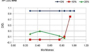
Fig. 9. Relative changes in smoking engine as a function of the relative load changes for different fuels at a rotational speed 1200 rpm
