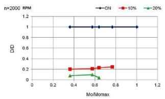
Fig. 11. Relative changes in smoking engine as a function of the relative load changes for different fuels at a rotational speed 2000 rpm
