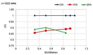
Fig. 4. Relative changes in the overall efficiency of the engine as a function of the relative load changes for different fuels, for speed 1600 rpm
