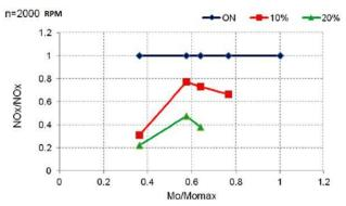
Fig. 8. The relative changes in concentrations of NOx in the exhaust of the engine as a function of the relative load changes for different fuels for rotational speed 2000 rpm
