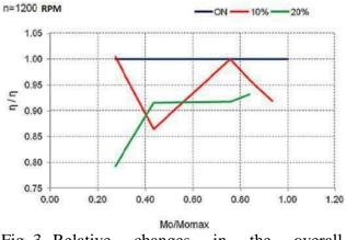
Fig. 3. Relative changes in the overall efficiency of the engine as a function of the relative load changes for different fuels, for speed 1200 rpm
