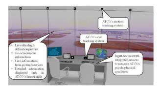
Figure 9. The basic set-up of the overall system.
