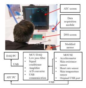
Fig. 7. Use of the developed mouse with micro sensors (DAQ- data acquisition board, MCU – Micro controller unit, USB – universal serial bus, DSS – decision support system)
