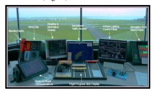
**Fig. 5. ATCO workstation at a relatively small airport** (Ronaldsway Airport, Island of Man , photo: Jon Wornham - http://www.island-images.co.uk/ATC/zRon2014/1009221616.html)
