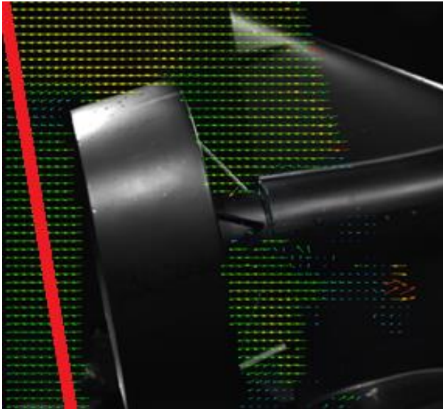
Fig. 3. An exemplary velocity field (free-wheeling fan, \alpha=10^\circ ) and the line of outflow velocity distribution
