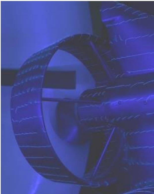
Fig. 7. A tuft visualization for windmilling fan, \alpha=10^\circ . A flow separation appears on the upper fan of the duct
