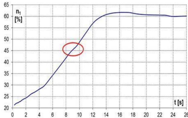
Fig. 8. Change in the rotational speed of the engine during start-up of the SO-3 type engine during the flight (much lower collapse of rotational speed growth visible)
