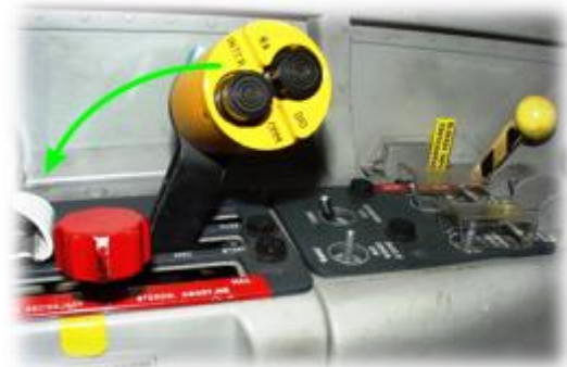
Fig. 2. View of the power lever (a green arrow – direction of lever movement)
