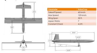
Fig. 11. 2015-16 design team final design of an AUAS to meet RFP requirements
