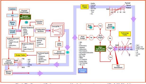
Fig. 1. The Conceptual Design process used by design teams (courtesy of Dr. L.M. Nicolai)
