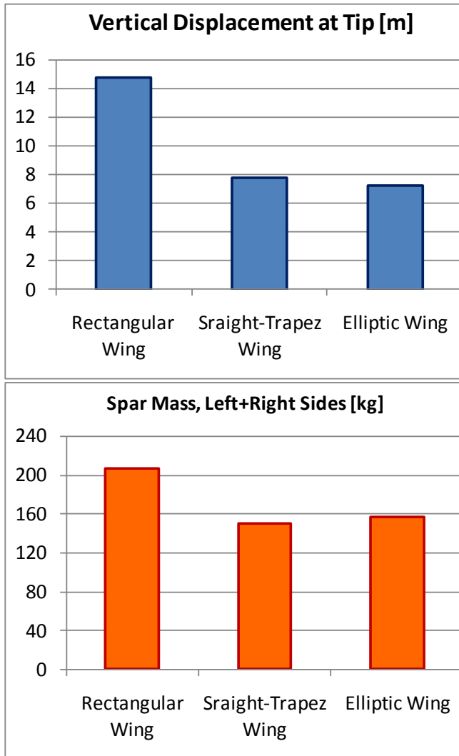
Figure 14 – Comparison between Rectangular, Straight Trapezoidal and Elliptic Wings
