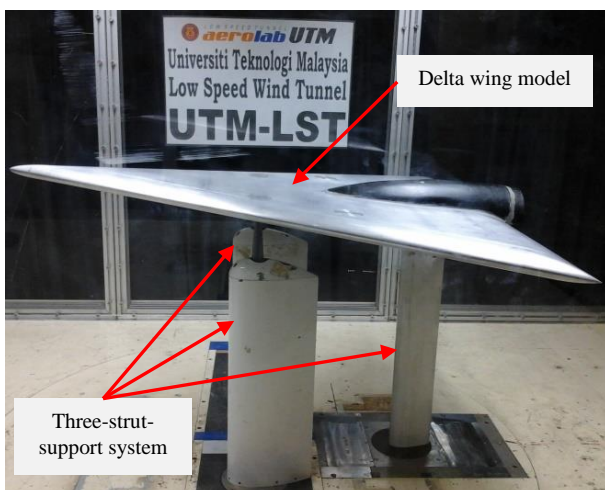
Fig. 1. Installation of UTM-VFE2 model in UTM-LST
