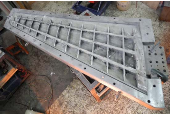
Fig. 7 The scaled model in hand lay-up process
