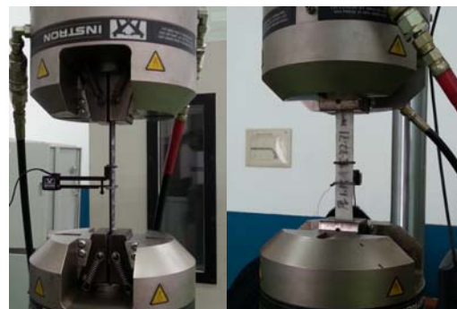
Fig. 2 The tensile test of the composites material
