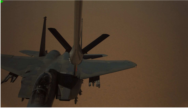
Figure 1-1: A330 MRTT vs F15 pair to pair qualification
