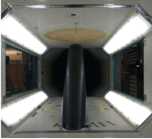
Figure 12 Experiment on the swept wing NACA 0050.
