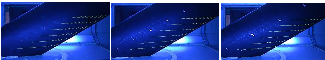
Fig 13: Flow visualisation over the rear end of the model using fluorescent tufts and UV lighting comparing the clean wing (left), \delta/h_v=1 (centre) and \delta/h_v=0.63 (right) with D/h_v 18 at x/c 0.5 and \beta = 30^\circ .
