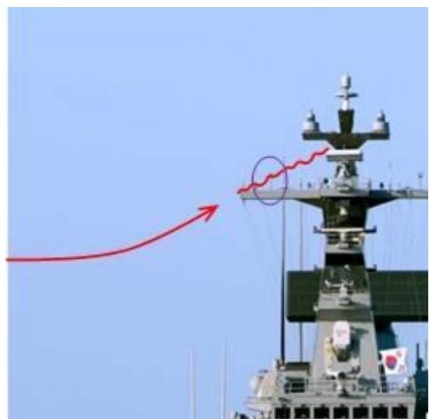
Fig. 15: Upwind anemometer in turbulent wake from yard.
