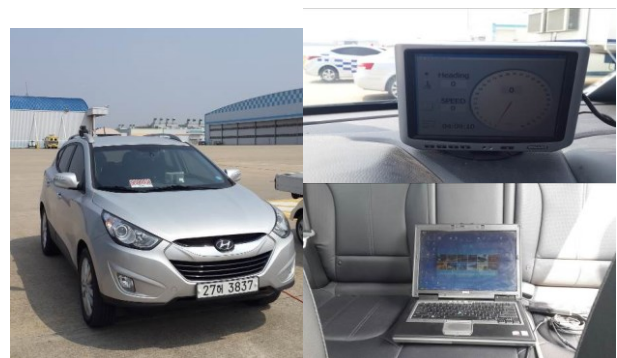
Fig. 5 Pace car (left picture), display for pace car driver (right top picture) and data processing and recording system based on a laptop computer (right lower picture).
