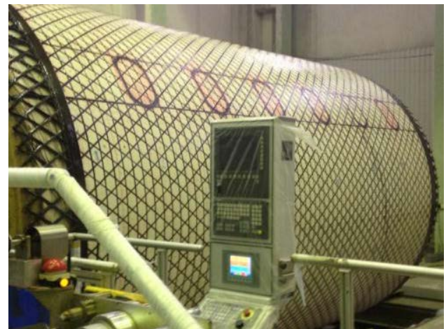
Fig. 4 – Winding of lattice composite fuselage barrel (CRISM)
