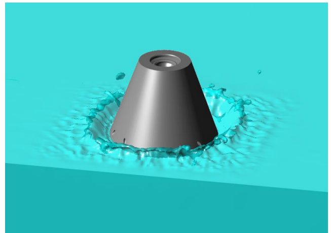
Fig. 10. Free falling case of REV splashdown. Water distribution
