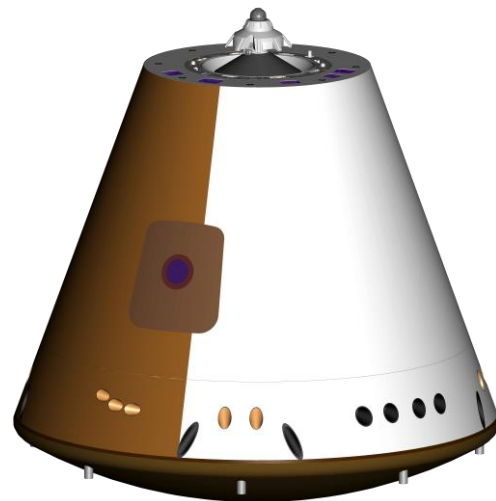
Fig. 1. Reentry vehicle of a manned transportation spacecraft
