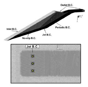
Fig. 3. Computational Domain and Boundary Conditions.
