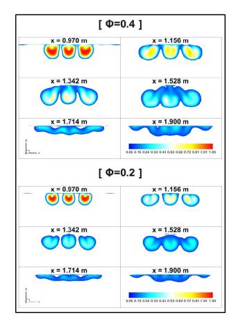
Fig. 7. Comparison of Ethylene Mass Fraction Contours between Different Equivalence Ratios.
