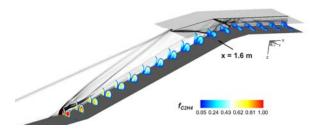
Fig. 4. Density Gradient Magnitude Contours at Mid x-z Plane and Ethylene Mass Fraction Contours at Several Cross-sectional y-z planes.
