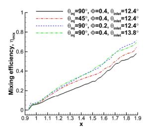
Fig. 5. Mixing Efficiency Comparison for Varying Injection Angle, Equivalence Ratio and Inlet Ramp Angle.
