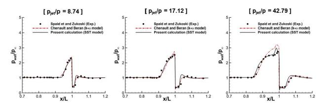
Fig. 1. Comparison of Surface Static Pressure Distributions for Spaid and Zukoski's Configuration [12].
