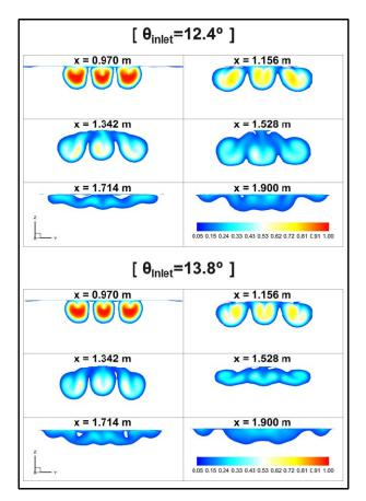
**Fig. 8.** Comparison of Ethylene Mass Fraction Contours between Different Inlet Ramp Angles.
