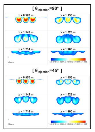
Fig. 6. Comparison of Ethylene Mass Fraction Contours between Different Injection Angles.
