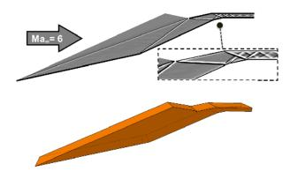
Fig. 2. Two-dimensional Shock Pattern (top) and Three-dimensional Geometry (bottom) of Inlet.
