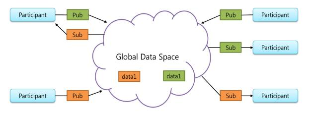
Fig. 1. DDS communication model
