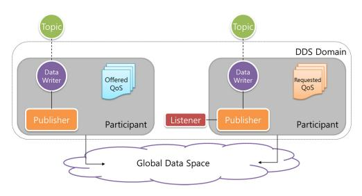
Fig. 2. Object model for DDS
