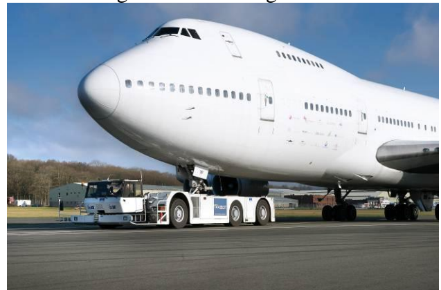
Fig. 1: TaxiBot towing a wide-body aircraft [7]
