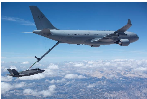
Figure 1: Refuelling operation with the flying boom system with an A330 MRTT (tanker) and an F-35A Joint Strike Fighter (receiver)
