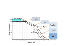
Fig.15. Conversion Corridor of 40% Small scaled Flight Demonstrator
