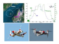
Fig.1. Flight Trajectory and Speed & Altitude of Smart UAS Flight Test (One hour Flight with Max. Speed of 440km/h at 3km Alt.)
