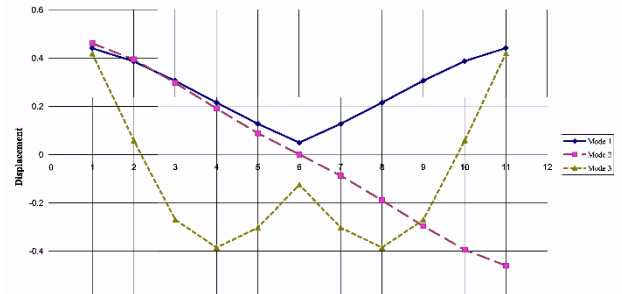
Fig. 8. Numerical simulation – 11 DOF system, first 3 normal modes
