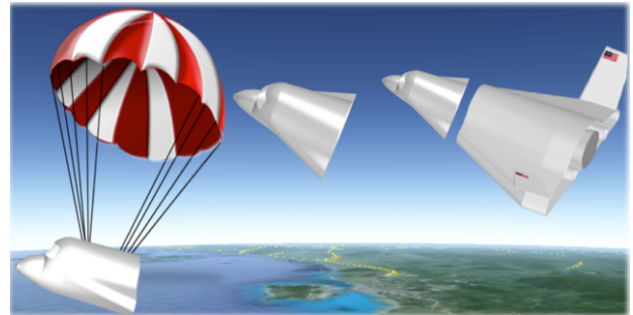
Fig. 8 Un-powered gliding in case of emergency during re-entry and descent
