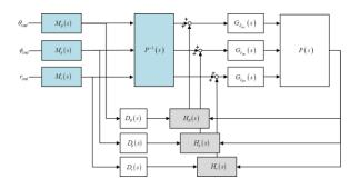
Fig. 2. Model Following Control(MFC) system
