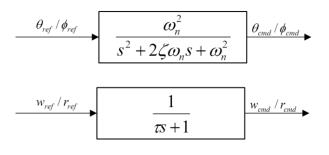
Fig. 3. Command model (up: pitch/roll, down: yaw / heave)
