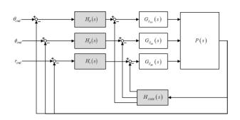
Fig. 1. PID control system
