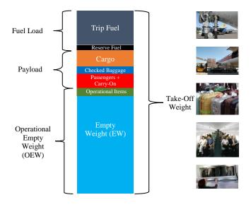
Fig. 1: Aircraft take-off weight breakdown.
