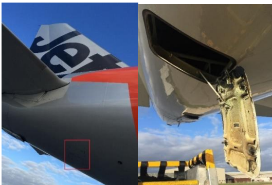
Figure 4: Location of access hatch on A320-200 aft of the rear pressure bulkhead
