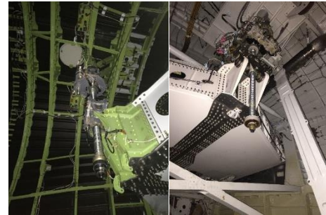
Fig 5: Elevator trim screw jack. Left 787-8. Right A320-200
