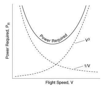
Fig. 7: Typical Airplane Power Curve
