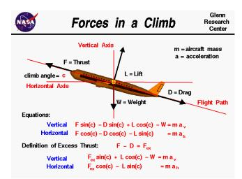
Fig. 6: Forces in a Climb – Source: NASA
