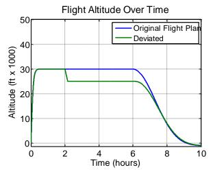
Fig. 4: Simulated Altitude Curves
