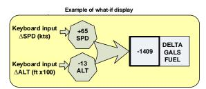
Fig. 2: A possible Display for Flight Crews and AOC to Evaluate What-if Scenarios
