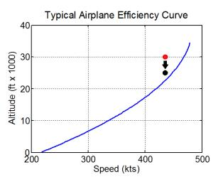
Fig. 8: Typical Airplane Efficiency Curve (derived from the power curve)
