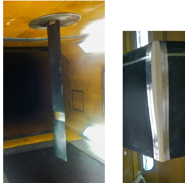
Figure 11. The baseline (zero cant angle) wing in the 8x6 wind tunnel working section (left) and an example of the foam inserts used at the fold-line to 'blend' the junction (right)
