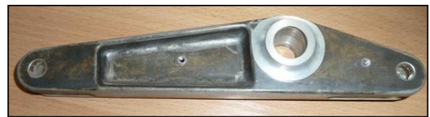
Figure 5: AZ31 magnesium alloy control – system lever
