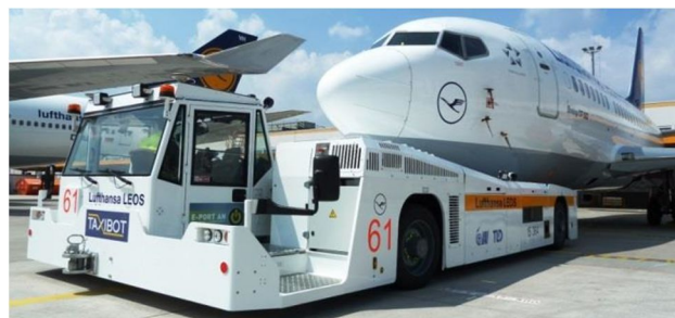
Fig. 1. TaxiBot towing a B737-500. [Source: Lufthansa LEOS]
