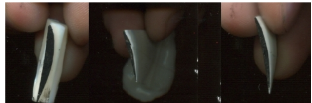
Fig. 4. The cross-section of the blades (bottom, middle and top profile of the blade)
