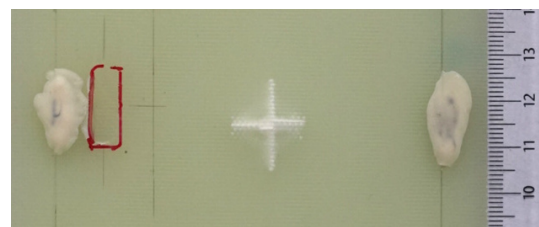
Figure 2: Impact damage (white cross).
