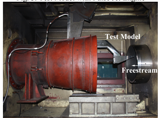
Fig. 4. Model Setup in FD-07 Wind Tunnel
