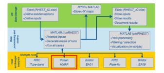
Figure 9, RHEST interfaces and data flow.
