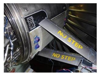
Figure 5, SHAFAE panel type heat exchanger
