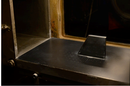
Figure 2. The flat plate with blunt fin model fixed in the wind tunnel test section
