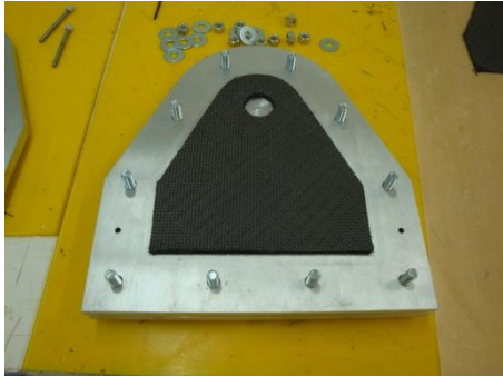
Figure 16. Mold assembly and positioned layers.
