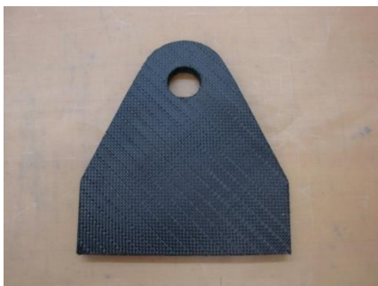
Figure 17. Preform manufactured on dry layers.
