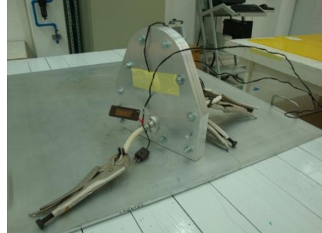
Figure 21. Mold assembly injected with resin prepared to curing process with thermocouples.
