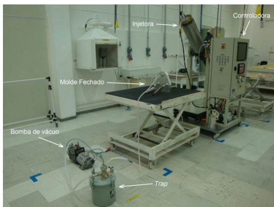
Figure 20. Injection system assembly of specimens.
