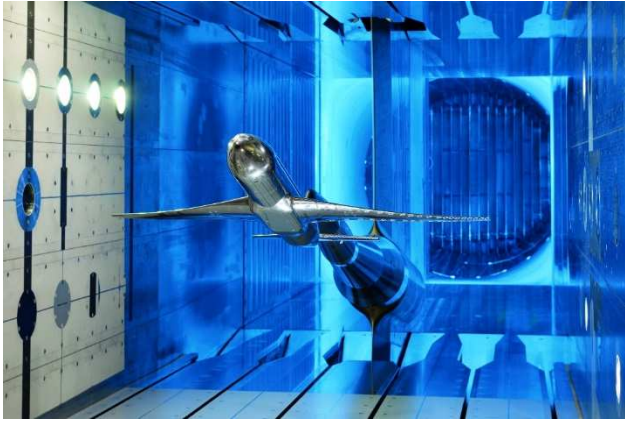
Fig. 2 CRM configuration in the ETW wind tunnel showing model and blade sting support
